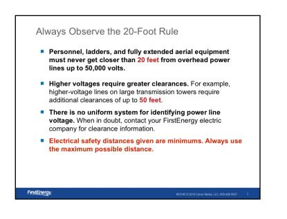
Always observe the 20-foot rule. The minimum safe distance from overhead power lines is 20 feet.
